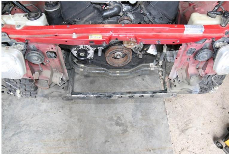
4. With the radiator in place it is now time to drill new 12mm holes thru the core support and radiator flange. Once the holes are drilled you can bolt the radiator in place. The radiator mounting flange may sit slightly out from the core support at the bottom. You can put rubber isolator pads between the flange and core support to eliminate this gap and provide a cushion for the radiator against the core support.
