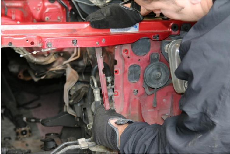
2. Now it is time to remove the front of the core support cross brace. You will need to cut the brace far enough back so as to create enough room for the radiator to sit in its place. Usually trimming back to the width of the new core support hole is enough. If you want something cleaner you can remove spot welds and pull the whole brace out.
